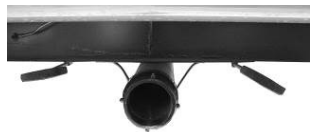
Black/Grey Tank Drain & Valves
