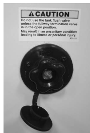
Tank Flush Inlet
